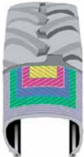
Radial tire construction: The cords are placed towards the tire center with 90 degrees.
